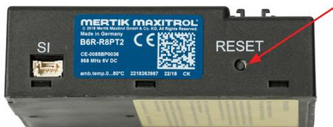
You now have 11 seconds to press the arrow down button on the remote control. Hold the button in until you hear a short "beep" from the receiver. You will know see the world "conn" on the remote control.
