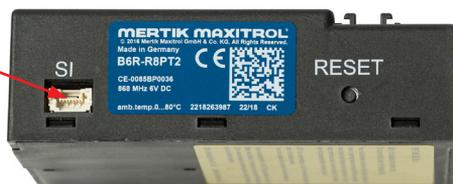
The wide connector on the wi-fi cable should be connected to the MyFire wi-fi-box.
