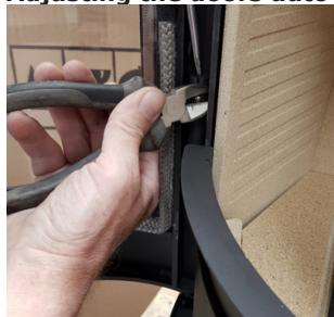
Remove the split and tighten the screw (clockwise) depending on how fast the door should close.
