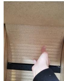
**3:** Once the top baffle plate from instruction 2 has been lifted, the upper vermiculite back plate can be lifted across the tertiary beam.
